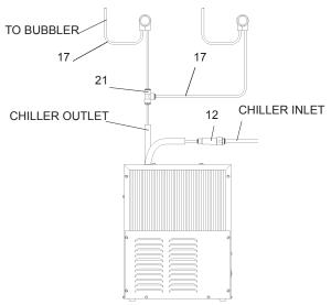
Figure 15 - HRFSER/HRFESR Tube Routing
