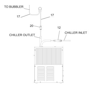
Figure 19 - HRFER/HRFSR Tube Routing
