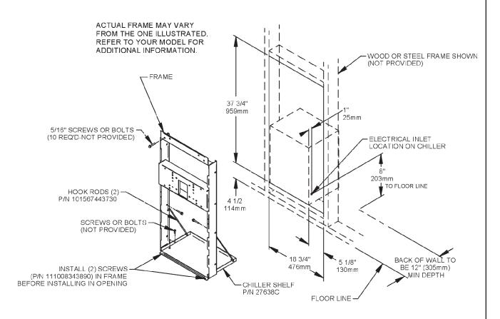
Figure 9 – Rough-In Assembly Single-Station Mounting Frames
