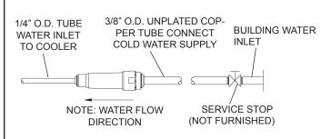
Figure 4 - Water Supply Connections
